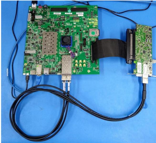
Fig. 1. SpaceFibre Endpoint Performance Test System
