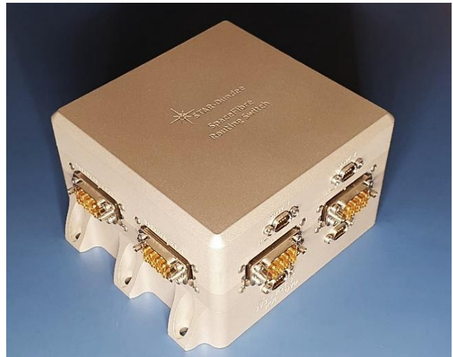
Figure 6: STAR-Tiger SpaceFibre Routing Switch
