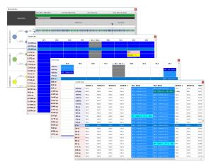
The packet and symbol views have **built-in search capabilities** to help navigate and validate captured traffic. If required, the data can be exported to a CSV file for custom software to interpret.
