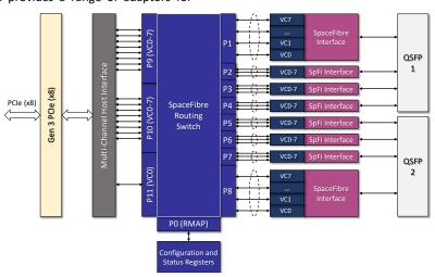
**Eight SpaceFibre single-lane interfaces:** Fully compatible with the SpaceFibre standard (ECSS-E-ST-50-11C). Lane data signalling rates configurable up to 6.25 Gbit/s are supported.
