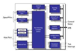
The IP core comprises a number of serial SpaceWire interfaces or optional parallel host port FIFO interfaces which are interconnected via a non-blocking wormhole packet switch. The packet switch implements address decoding for both path and logical address, output port arbitration, and packet routing.
